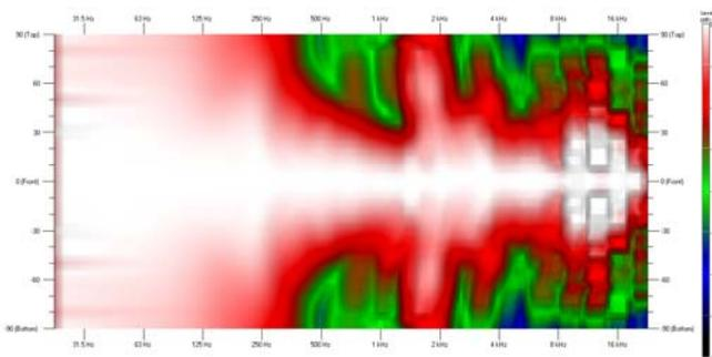
Figure 16: Directivity map of a real loudspeaker system response with measured data of the individual acoustical sources
