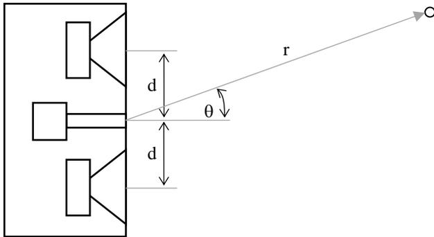
Figure 1: Geometry of example loudspeaker system
