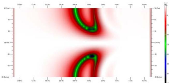
Figure 4: Directivity map of system with 1.2 kHz, 4th order Linkwitz-Riley crossover
